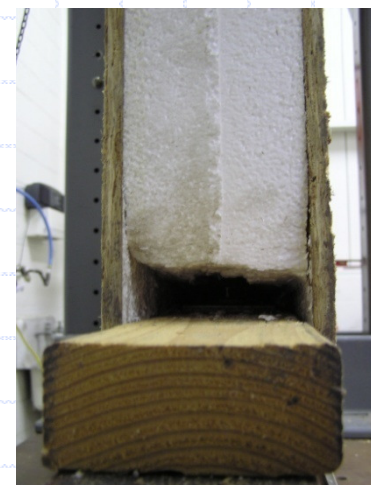
EPS core crushing
